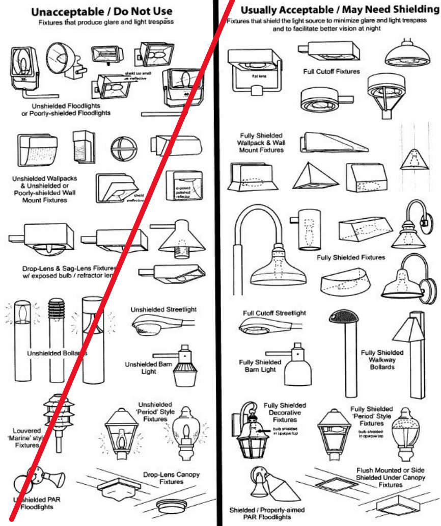
Figure C: The lights on the left are nonconforming. Those on the right can be used in most cases. However, the mounting height and proximity to the property line may cause the lights to need additional shielding to prevent the luminous elements from being visible from any other property. 4. Nongovernmental light fixtures, if rated by the B-U-G classification system:
